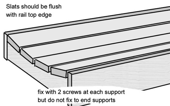
After sanding and smoothing off any sharp edges, evenly space the seat slats and fix them to the four innermost seat supports only. Use two screws at each spacer junction. Don't fix slats to either of the end supports
