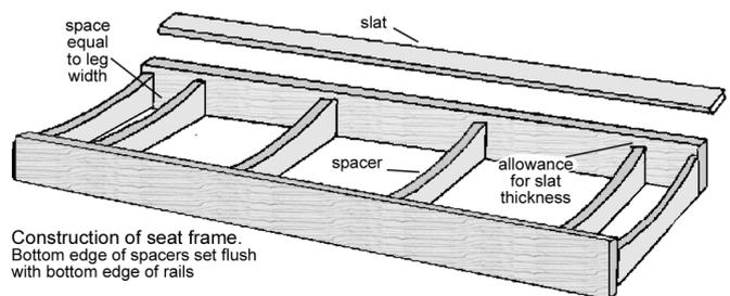
Now take the second and second last seat supports and fix them to the top rail. The spacing should be the width of the leg material. You could use an off-cut of one of the legs to set the spacing.
