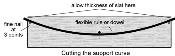
The curve can be as gentle or steep as you like, but make sure that you leave enough "meat" to provide adequate support ... a minimum of 45mm is suggested if you are using 100mm x 25mm (nominal) timber. Drive in a fine nail at each of the points and using a flexible ruler or piece of fine dowel, bend it around the nails and then draw your curve using the ruler or dowel as a guide.
