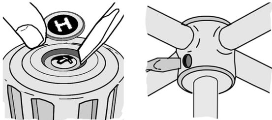
Remove the flange (and spring, if fitted). Some traditional type taps have a flange that needs to be unscrewed by hand or with multi-grip pliers. If using multigrips, wrap a cloth around the shield first so that the jaws won't damage the surface. When the flange is unscrewed, move it up the handle to expose the tap body.
