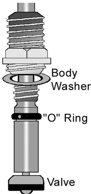
If the tap has been leaking from beneath the flange at the base of the tap, it is a worn body washer (usually a red fibre washer at the base of the spindle) and you can lift it off and replace it with a new one.
